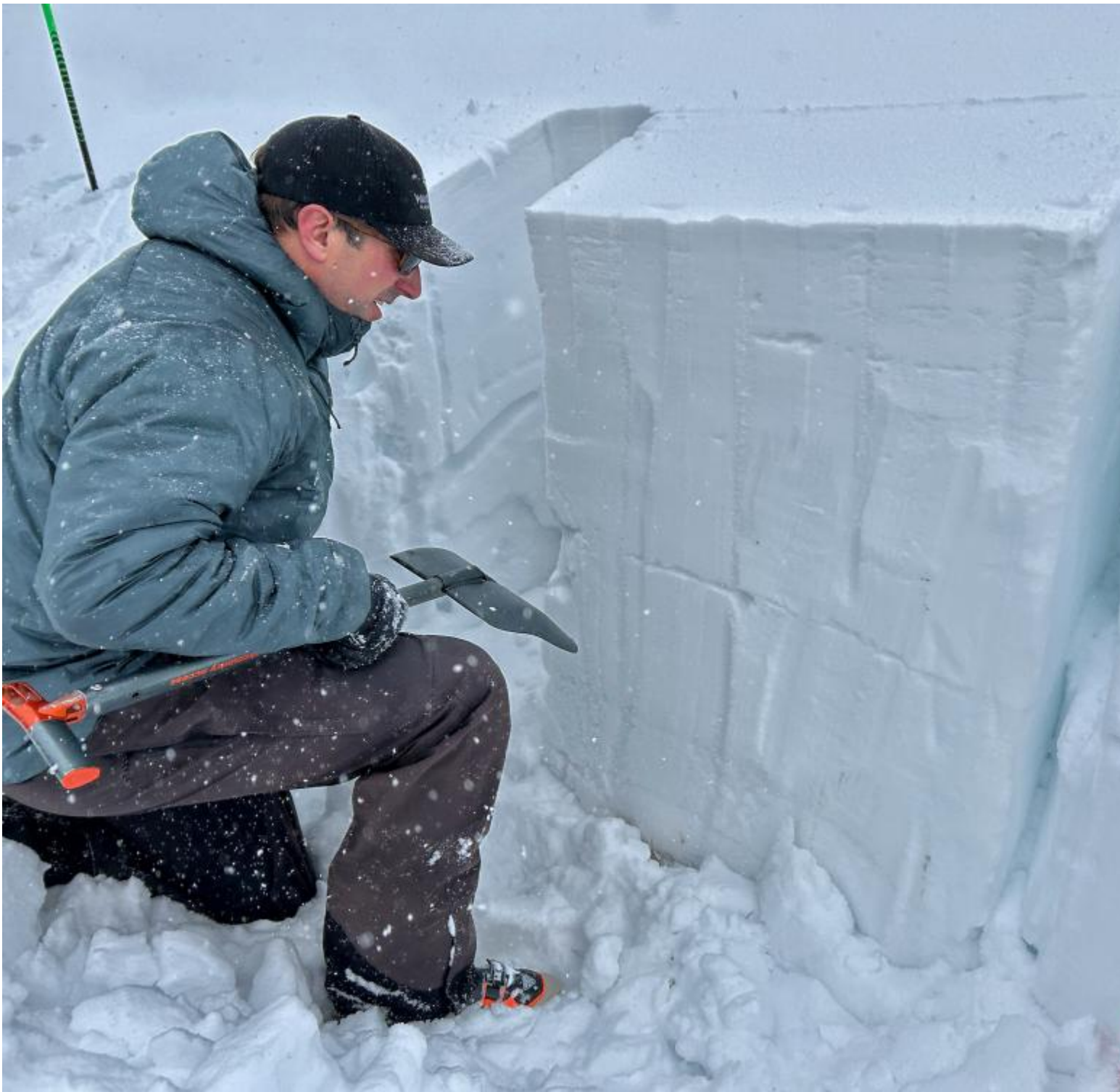
Divide Pk 9560ft E facing snowpit, ECTP30 about 24" deep on 27 Dec 2024
