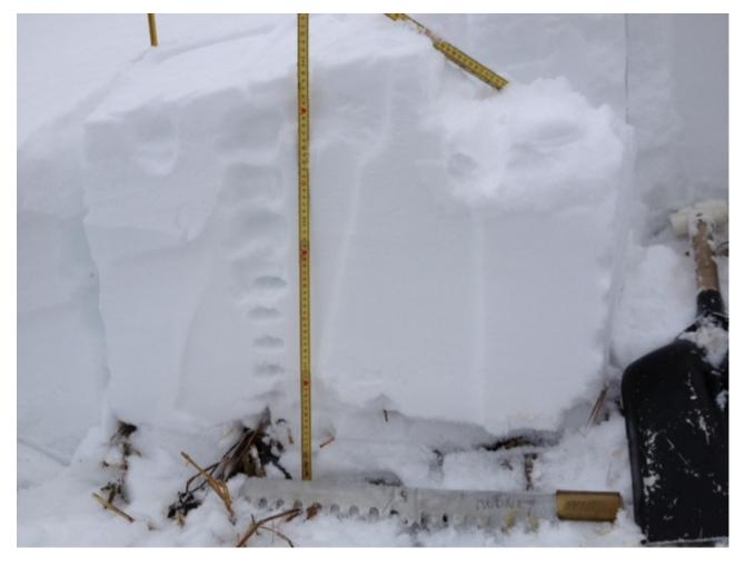
Bridger Bowl Snbow Safety dug this pit near the top of Pierre's Knob lift. They got collapsing on the layer of facets near the ground as they skied. Test score on the column were ECTP18 breaking 12 cm from the ground. Photo: P. Maleski
