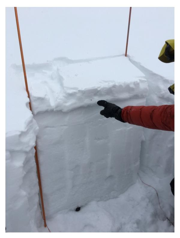
A 2" thick wind slab is cracking, whumphing and breaking easly in stability tests (ECTP3). This was seen in the Throne area of the northern Bridgers. Skiing and sledding was reported to be "awful" from the winds. Photo: B. Nobel
